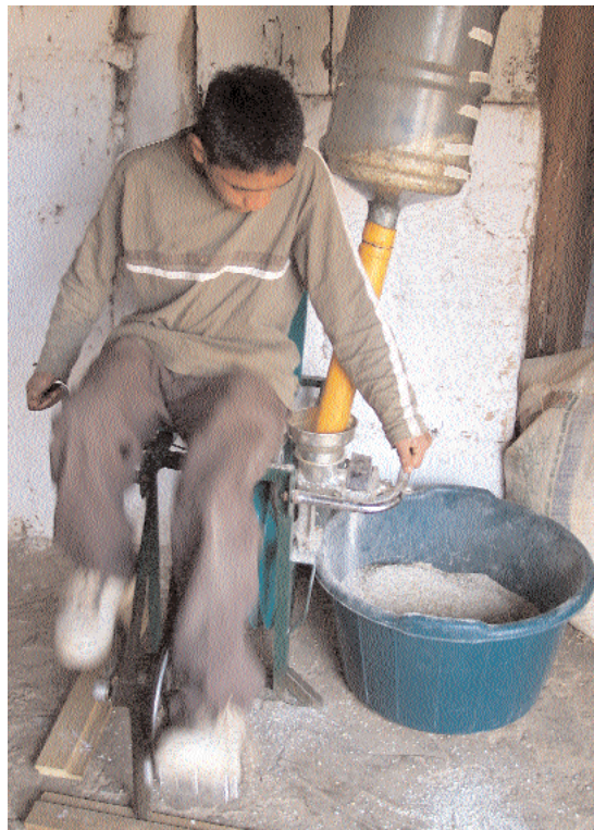
A man grinds corn using Maya Pedal's signature machine, a bicimolino.
